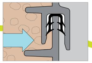
3-sided element seal (Triple-Safety-Seal) The only chamber element seal that seals inwards and outwards.
