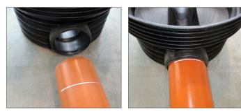
ckets. The connecting sockets are designed for direct fitting of PVC pipes in accordance with EN 1401, PP pipes in accordance with EN 1852 or plain plastic pipes. For the connection of other pipe materials, adapters or short pipes and cuffs should be used.
