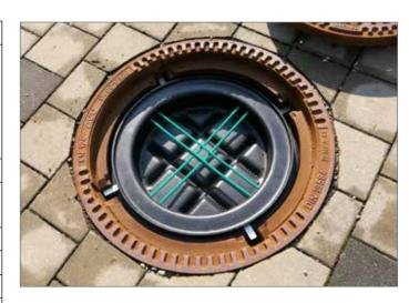
cover diameter. This is done using a size 13 mm spanner, which is used to loosen and countertighten the M8 nuts at the mounting brackets. These can be moved to adapt to the concerned diameter. The mounting brackets are factory-fitted for the smallest diameter of 595 mm. At least 10 mm of the brackets should fit flat. The distance between outer edges of the indentations in the cover should be measured before installation to allow the brackets to be precisely set.
